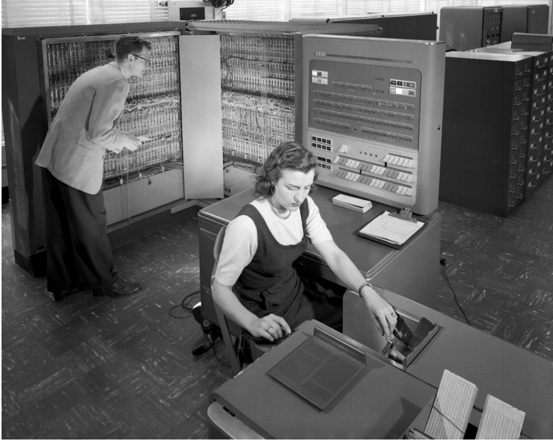
Man and woman working with IBM type 704 electronic data processing machine used for making computations for aeronautical research. By NASA, Public Domain
